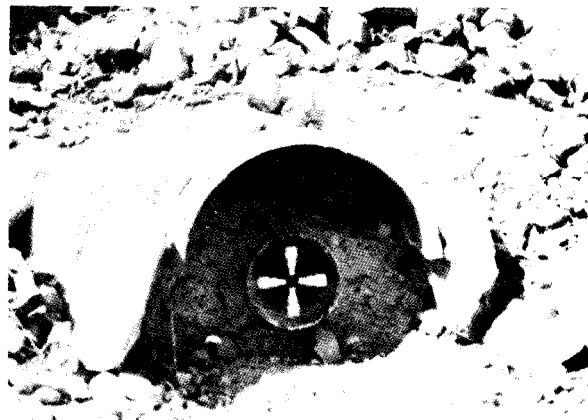
Figure 13-26. A reference sighting target for use in obtaining collimation measurements.—P526-400-7852
