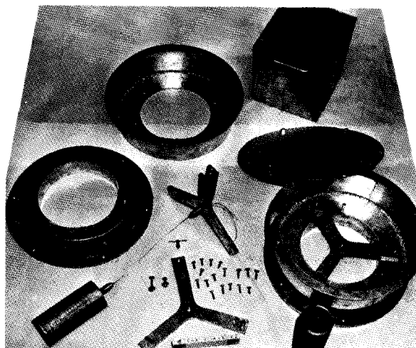
Figure 13-20. Components of equipment for weighted plumbline installation.-PX-D-74010
