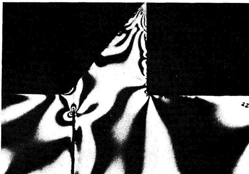
(b) FAULT SEAM EXCAVATED, BACKFILLED 52 FEET
