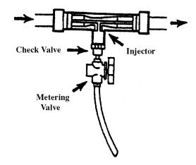
Fig. 2. Venturi device.
