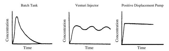
Fig. 1. Chemical concentration levels during injection using a batch tank, venturi injector and positive displacement pump.
