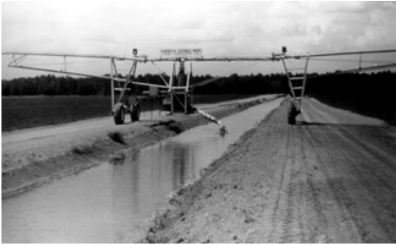
Figure 5. Ditch-fed linear move irrigation system
