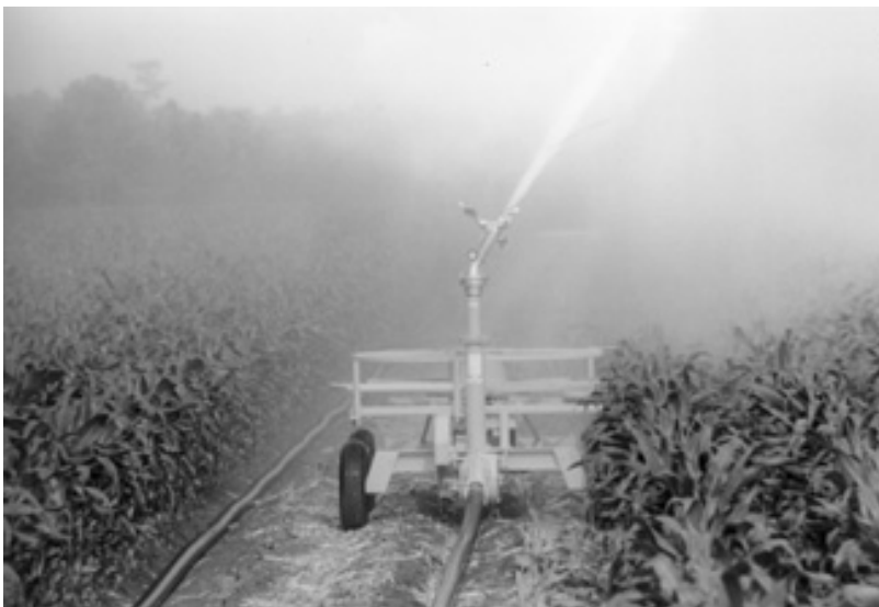
Figure 7. Cable-tow traveler irrigation system
