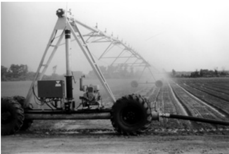
Figure 6. Hose-fed linear move irrigation system
