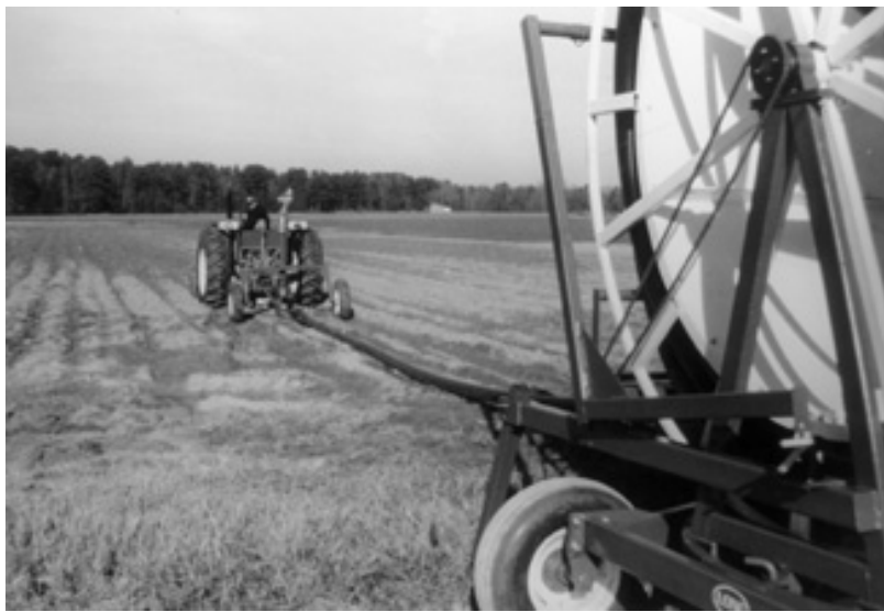
Figure 8. Hose-pull traveler irrigation system
