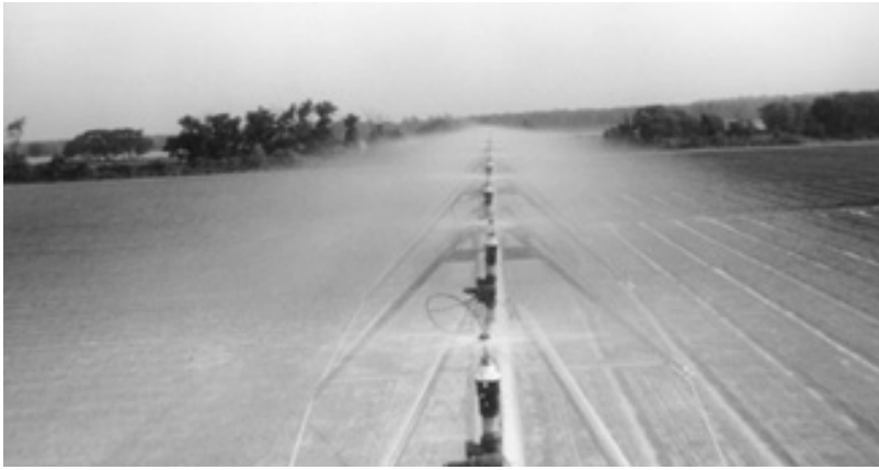
Figure 2. 360-degree spray nozzles with pressure regulators
