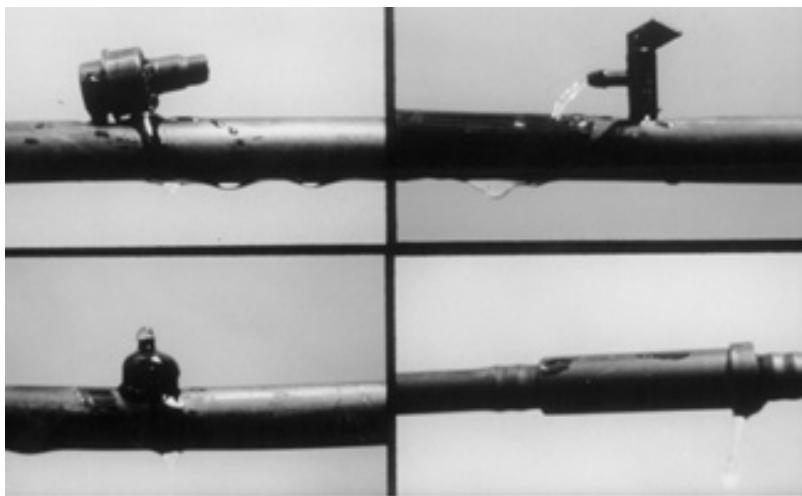
Figure 11. Examples of point source emitters
