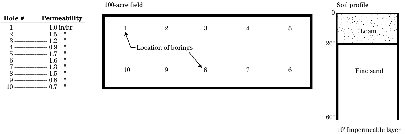
Figure 10-12 A field that requires few hydraulic conductivity tests (1 per 10 acres)*
