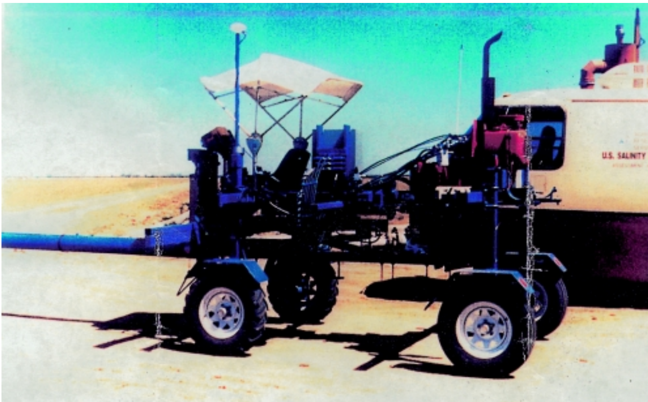
Figure 2 Combination, mobile electromagnetic-induction/four-electrode sensing system
