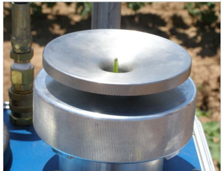
Figure 3. (Left) Plot showing the negative relationship between leaf water potential and the empirical crop water stress index using an artificial wet reference. Temperature and in situ measurements were made at mid-day during the 2007 growing season. (Pictured above) pressure chamber for measuring stem leaf water potential.
