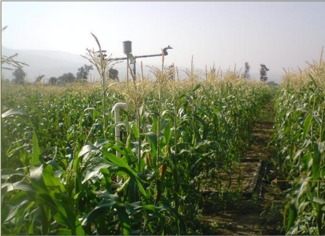
Figure 5. The weighing lysimeter with a sweet corn crop near harvest. The micro-meteorological equipment is on a mast (center left); and one edge of the lysimeter surface appears centered between corn rows (lower right).
