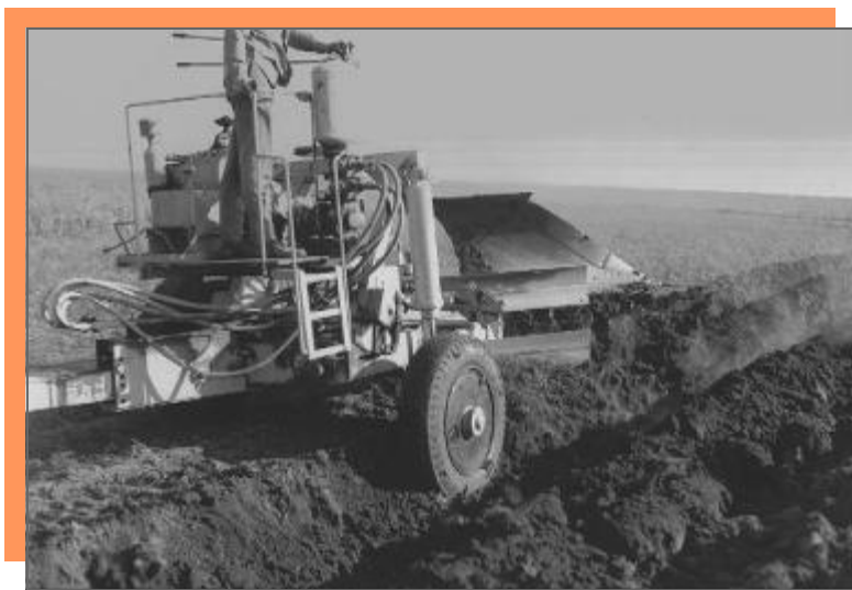
Fig. 1. Moldboard plow used to till conservation benches to 0.70 -m depth without inverting the soil. Plow was pulled by a D-8 Caterpillar tractor.
