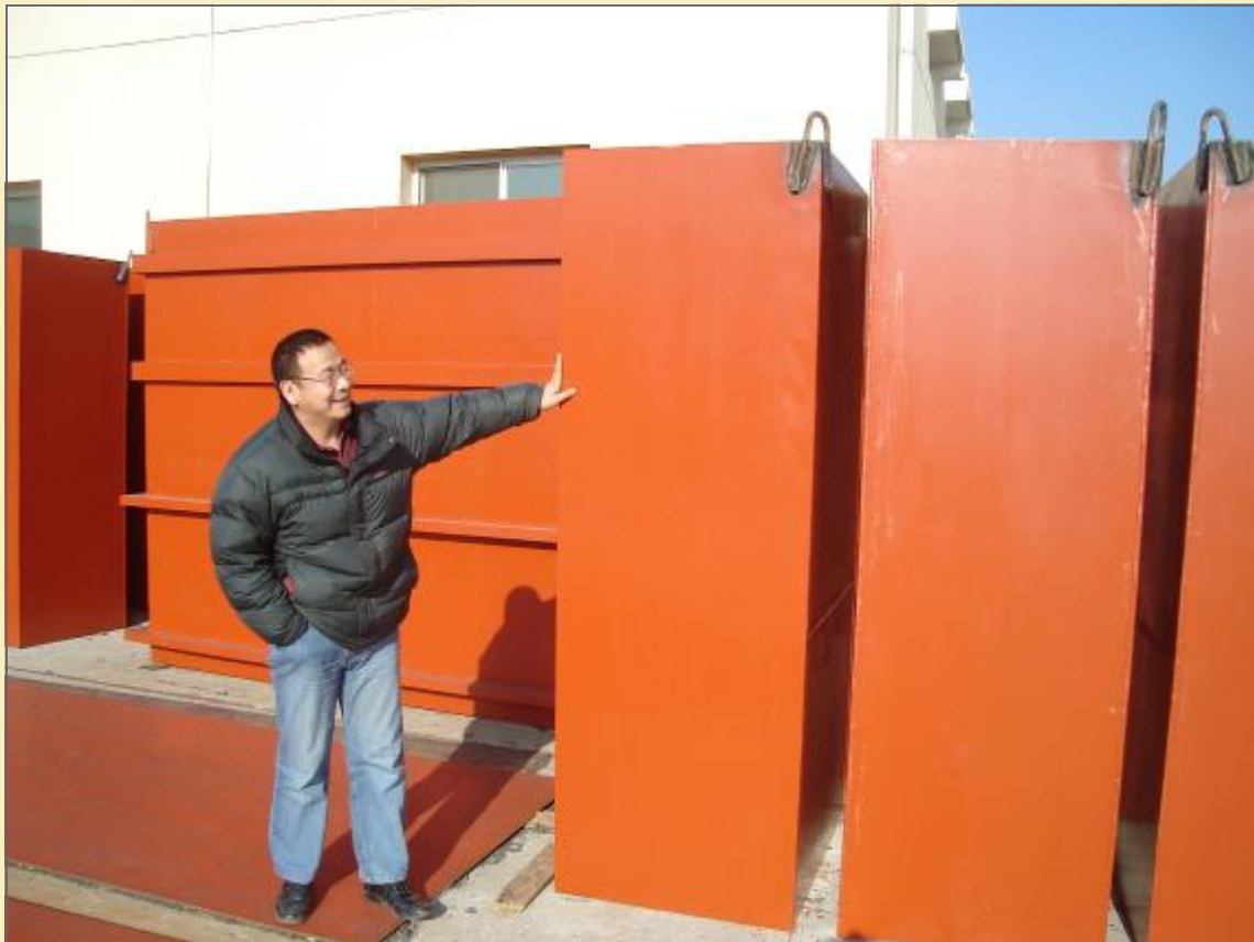
Figure 6. Dr. Xuzhang Xue with soil tanks for the large weighing lysimeter (behind him) and the smaller weighing lysimeters (he is touching one) to be installed at the research station of the National Engineering Research Center for Information Technology in Agriculture, Beijing, China.
