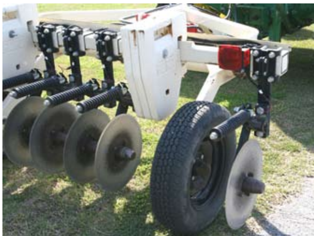
Figure 3 Georeferenced electrical conductivity equipment is used to develop soil texture maps
