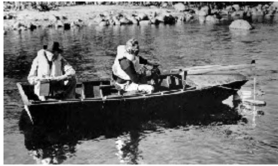
Figure 10-5 -- Making a current-meter measurement from a boat.
