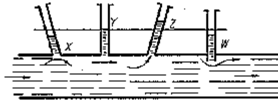
Figure 5-9 -- Examples of piezometer installation.
