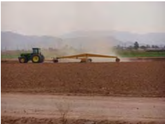
Figure 4-9 Field smoothing can be done by a land plane
