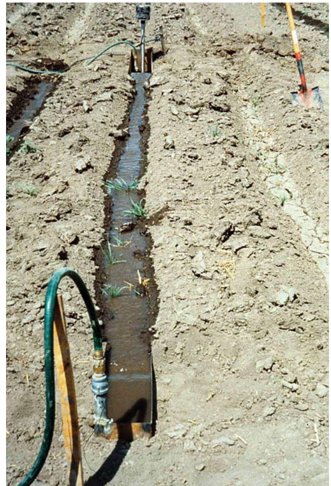
Figure 4-46 Flowing furrow infiltrometer
