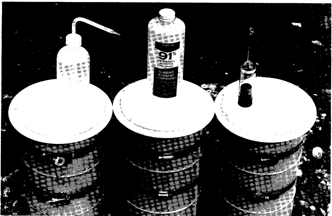
Figure 3-70.—Plastic squeeze bottle, isopropyl alcohol, and air indicator are used in determining the air content of freshly mixed concrete.
