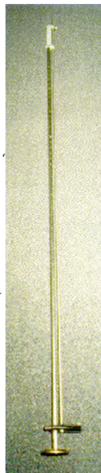
Figure 10-15 – Top setting wading rod.
