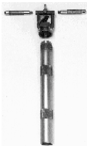
Figure 10-26 Hand-held sediment corer (courtesy Wildlife Supply Company)
