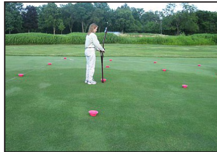
Figure 3. Sampling soil moisture with TDR300.
