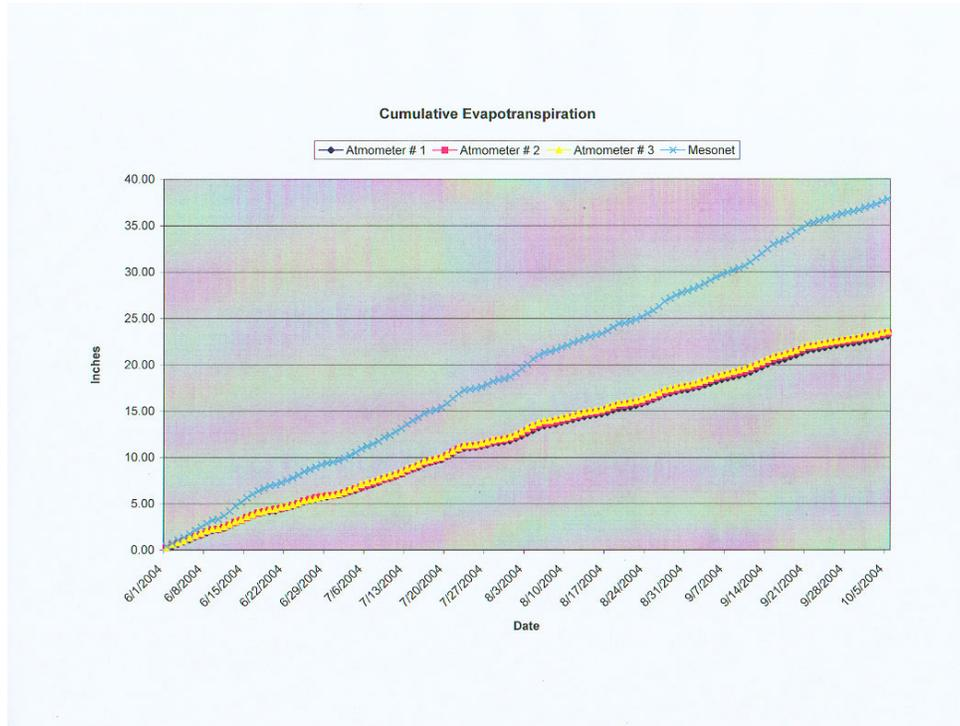
The results shown in Graph 3 indicated to NRCS that atmometers consistently provide accurate readings in comparison to each other when located at the same site. The results also indicated to us that an atmometer located in the same environment as an irrigators crop is a more valuable tool for scheduling than using readings from a remote weather station.
