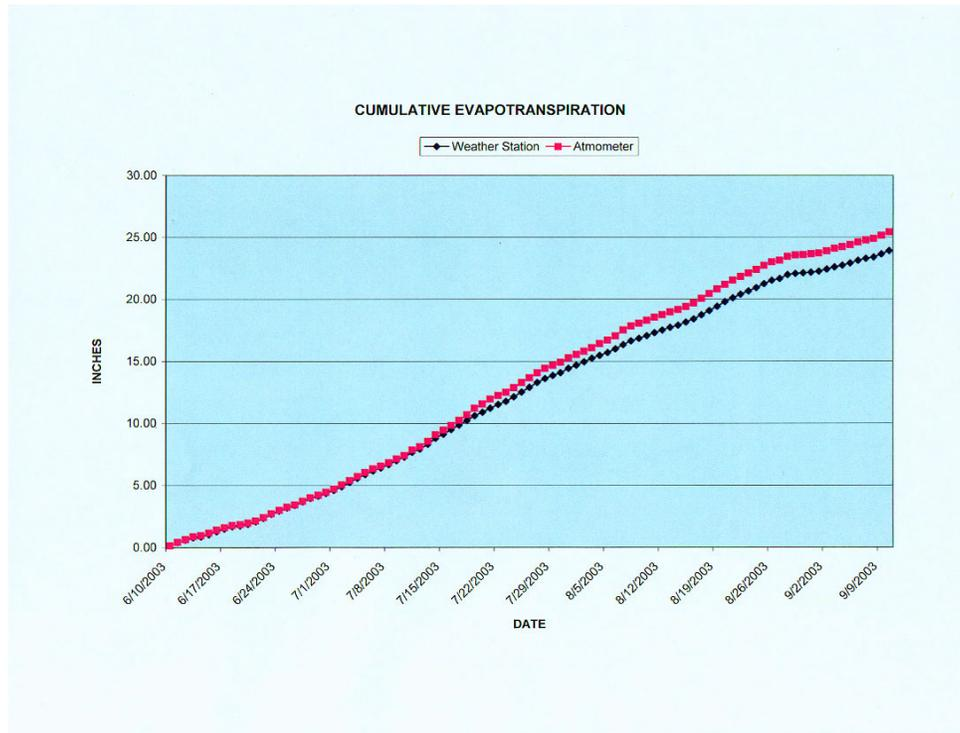
The field trial with OSU at Goodwell provided very similar results to the results in Graphs 1 and 2 above. The results in Graph 2 above indicated to NRCS that over a growing season, an atmometer can provide reasonable estimates of evapotranspiration similar to readings from a fully equipped weather station. Compared to a weather station costing thousands of dollars, the atmometer we found to be a simple and affordable device that could effectively be used by Oklahoma irrigators.
