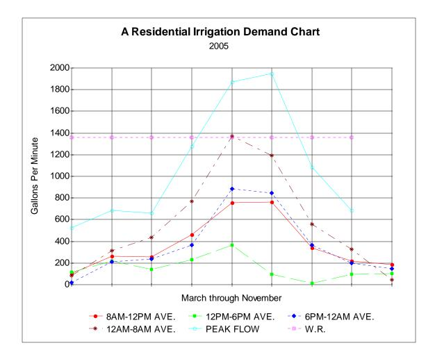
The area above and left of the peak pump line on the left half of the graph and the area above and right of the peak pump line on the right half of the graph indicate unused water. This constitutes about 25% of the annual water right.
