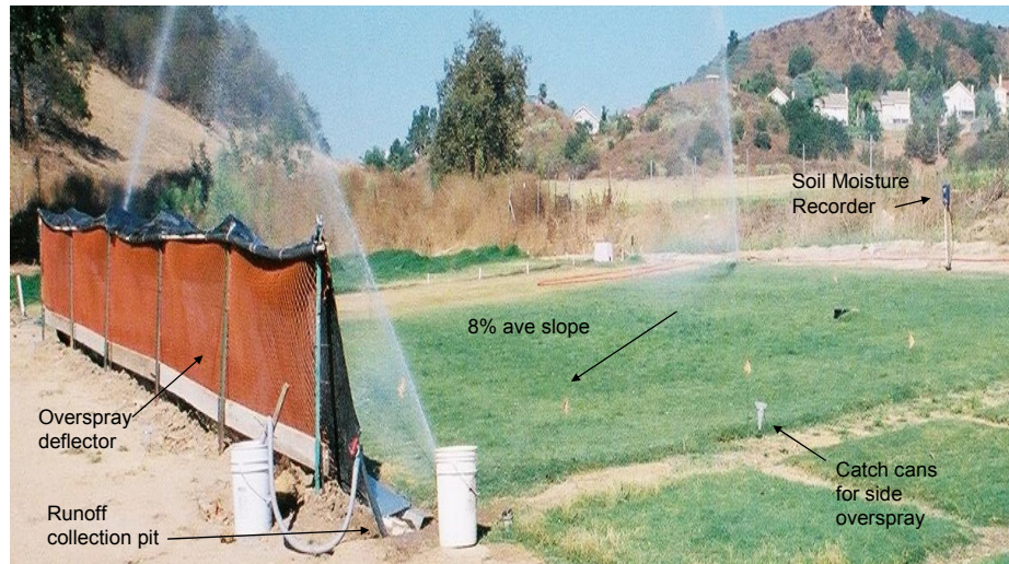
Figure 1. Layout of the irrigation runoff plots on a GN-1 hybrid bermudagrass turf with an 8% slope
