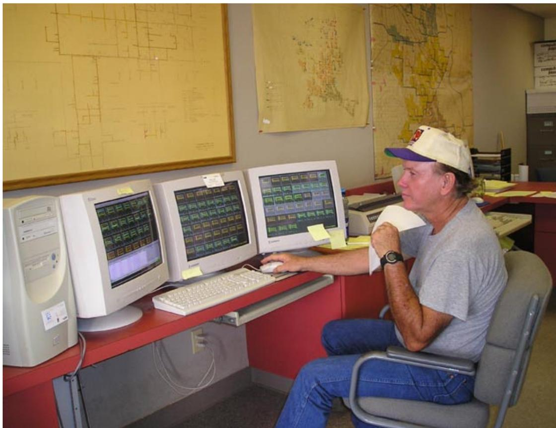
**Figure 3. An operator at the Central Arizona Irrigation and Drainage District (CAIDD) near Phoenix monitors primary flows and water surface elevations in the 60-mile canal. This SCADA system was implemented at relatively low cost using affordable RTU equipment and spread spectrum radios for communication.**
