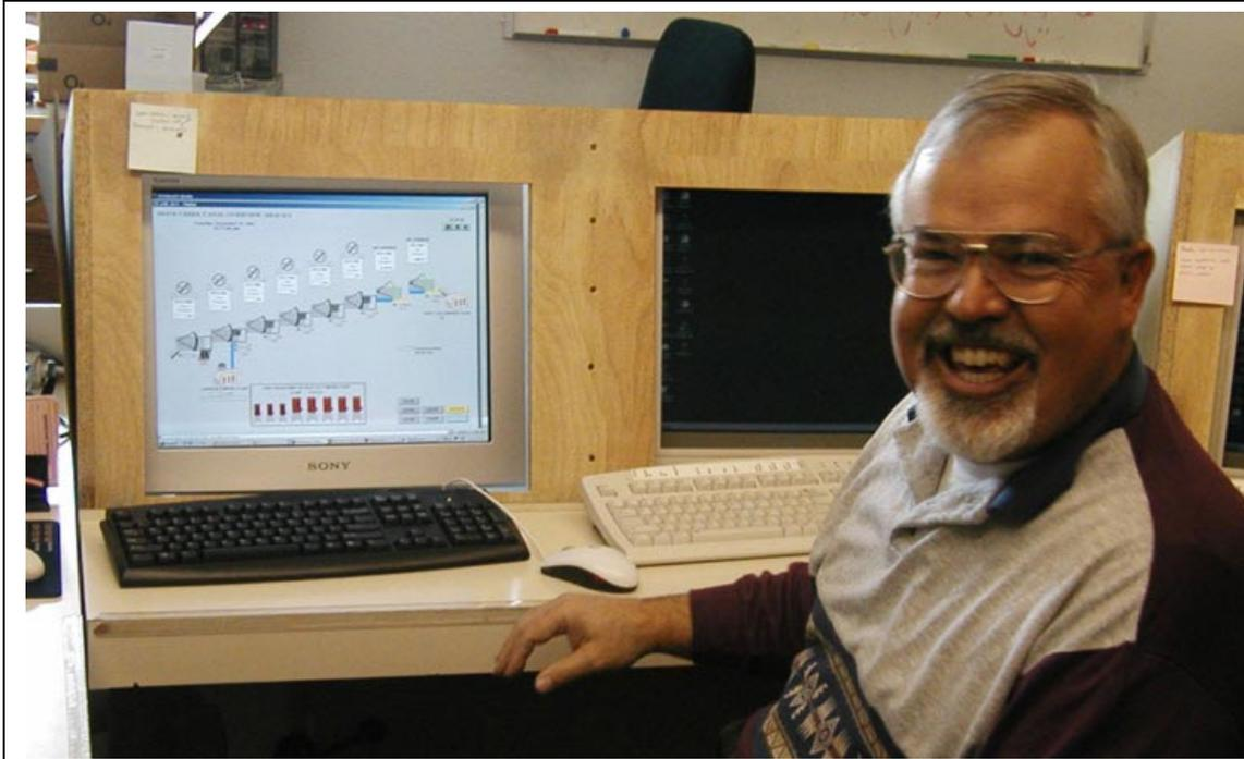
**Figure 2. Chuck Lurvey, district engineer for the Delores Project in Cortez, Colorado, is sitting in front of the SCADA central computer. Radial gate icons on the HMI screen indicate the water surface level in the canal and the gate positions of the radial gates at checks along the canal.**
