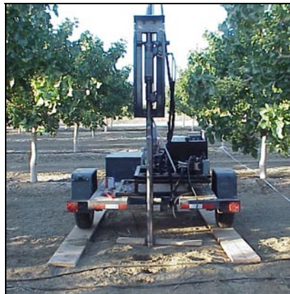
Figure 1. Soil core sampler in the field.
