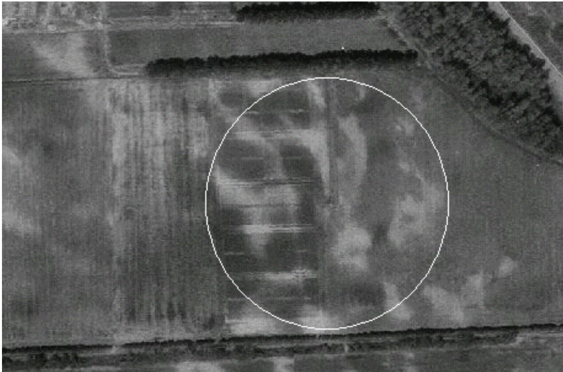
Fig. 1 Results of mapping apparent soil electrical conductivity ( EC_a ) with a Veris 3100 machine using the deep setting. Areas in the 0 to 5 EC_a range were grouped as one management group (SAND) and areas with values greater than 5 comprised the other group (SILT). The outline of the three pivot towers and overhang can be seen.
