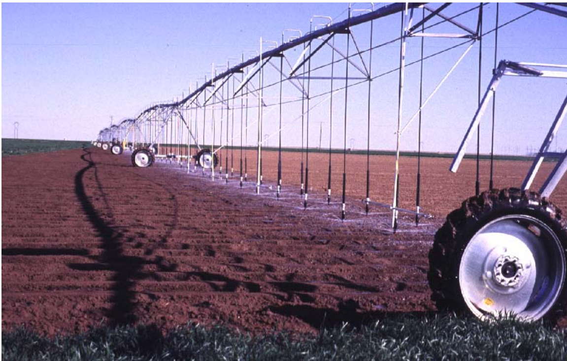
Figure 1. Typical example of a LESA system with spray heads on drops spaced 5 ft (1.5 m) apart). Note that the furrow arms and drop hoses alternate from one side to the other along the truss.
