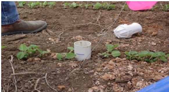
Figure 5.4. Installation of Sentek access tubes, clock-wise from upper left: 1) Tripod adjusted to the vertical, pinned to the ground, and with access tube inserted; 2) Lowering auger into tube from a ladder; 3) Tube nearly installed with horizontal mark that will be at soil surface when finished; 4) Installed tube with top cap; 5) Using a Giddings hydraulic push machine to push the tube 10 cm into the soil
