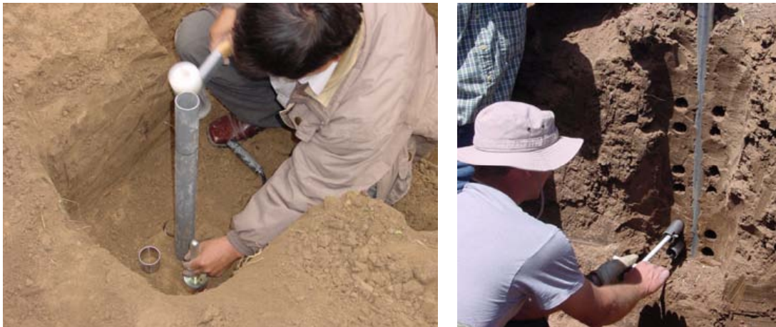
Figure 3.9. Two methods of obtaining volumetric soil samples during NMM calibration. In both photographs, a mark on the access tube indicates the original soil surface. Measurements are made downward from this mark to find sampling depths. (Left) Sampling with bevelled cylinders using a combination guide rod and holder. The centre of measurement is below the soil surface, which has been cut away so that the cylinders will be centred on that depth when they are inserted into the soil. (Syrdarya Branch Station, Uzbekistan; silt loam.) (Right) Removing Madera probe samples. The Madera probes were inserted horizontally, two just above and two just below the depth of the centre of NMM measurement, and as close to the access tube as practical. Two depths above have already been sampled. (USDA-ARS Laboratory at Bushland, Texas, USA; clay loam and clay.)
