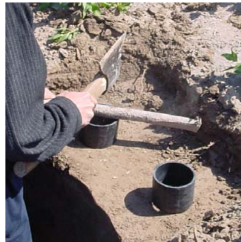
Figure 2.3. (Top) Bevelled volumetric sampling cylinders ( 100 \text{ cm}^3 ), one shown with plastic caps for sample retention (caps may not prevent water loss). (Left) Same cylinders during sampling around the access tube. One cylinder is shown fully driven into soil with no visible compression (top of left photo); another is shown resting on the soil surface prior to sampling; and a third is being driven into the soil with the cylinder holder/driver. (Right) A sampling cylinder made from plastic tubing is shown being driven incorrectly into the soil using a piece of wood as a hammering anvil. This method does not ensure that the force from each blow is transmitted directly down the axis of the cylinder. Off-axis force will cause the cylinder to tip downward on the side where the force is the greatest, causing the soil to shear at the cutting edge as the cylinder rotates.
