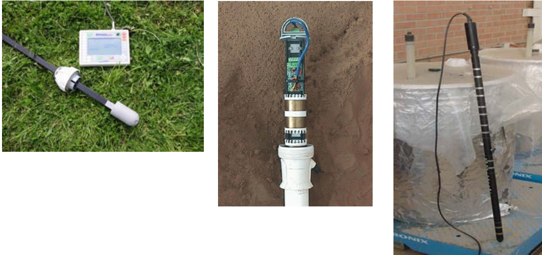
Figure 5.1. Examples of capacitance sensors: Sentek Diviner 2000 5 (above), Sentek Enviro-SCAN (right), and Delta-T PR1/6 (far right).
