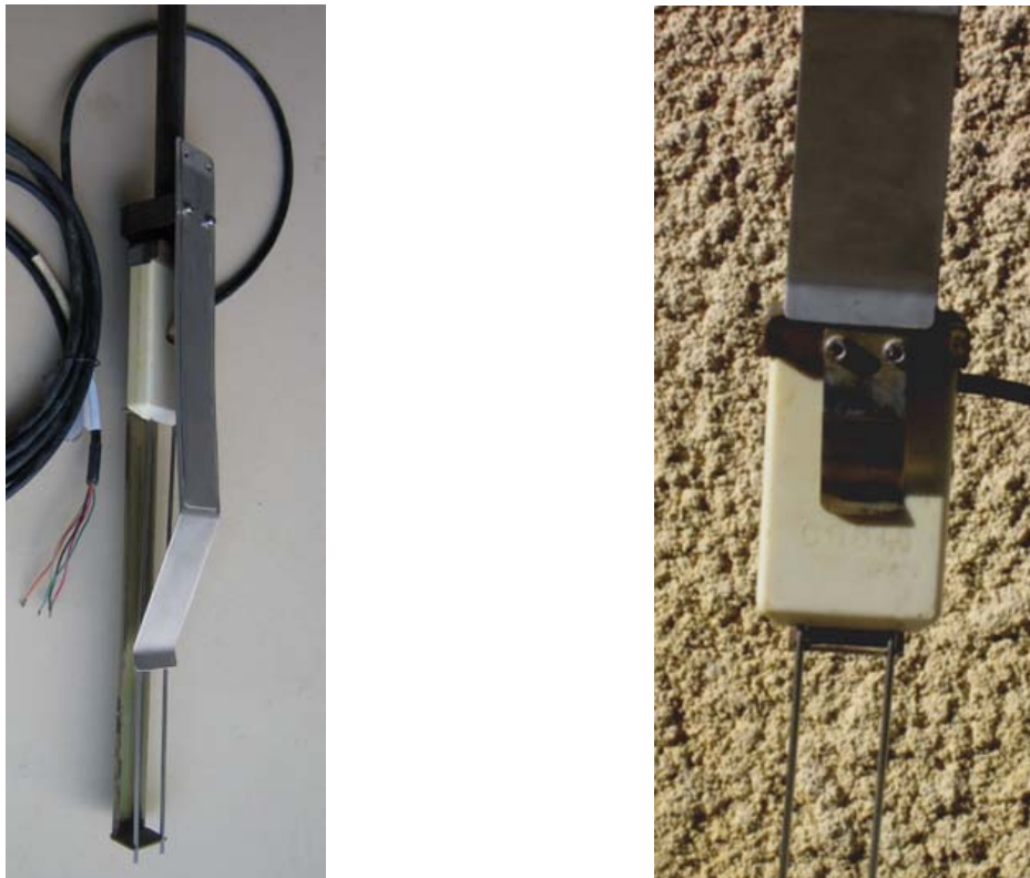
Figure 7.3. (Left) Insertion tool with a sensor to be pushed in the soil. The bottom end of the tool is notched to hold the probe rods the correct distance apart. (Right) Insertion tool to be taken off when the sensor is in the right position in the soil.
