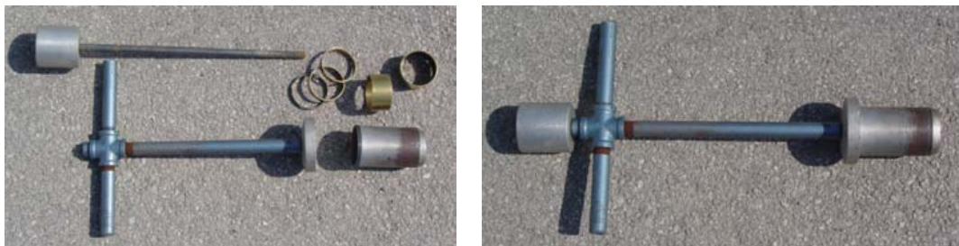
Figure 2.5. A slide hammer sampler that employs internal brass cylinders to contain the sample, disassembled (left) and assembled (right). The cross-sectional surface area of the cutting edge is easily twice the area of a directly driven bevelled cylinder as shown in Figs 2.3 and 2.4.
