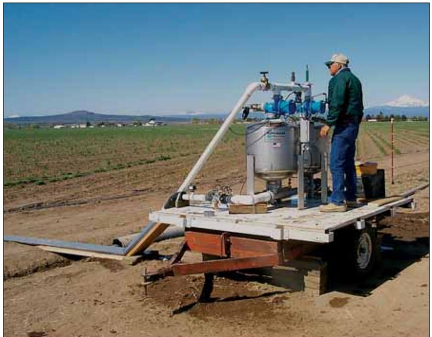
Figure 3.—Typical filter station, using two sand media filters, in central Oregon.
