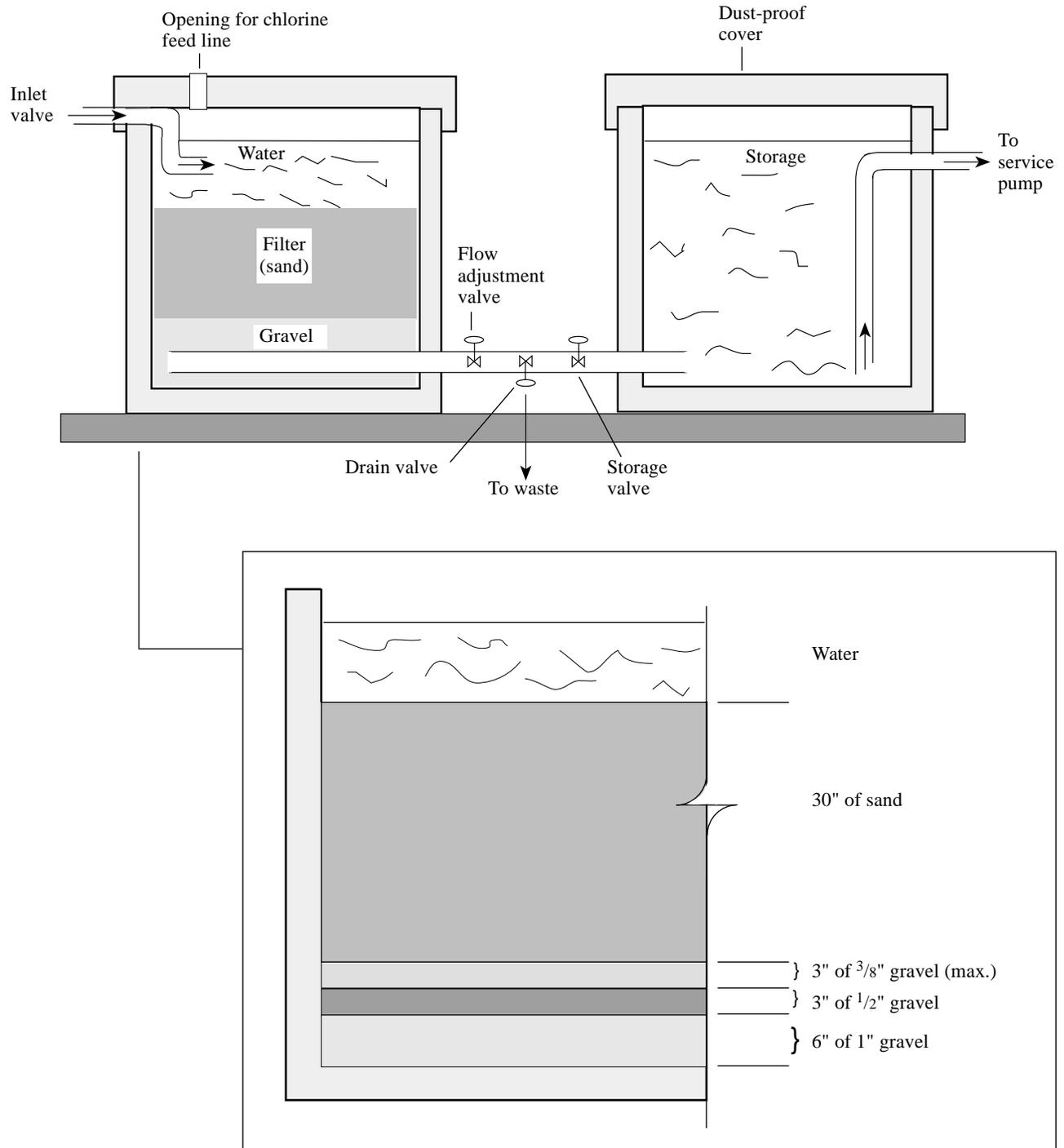
Figure 5.—An overall view (top) and a detail view of a constructed-in-place filter to clarify surface water. Based on a model in *Private Water Systems Handbook* (MWPS-14) by Midwest Plan Service, Ames, IA, 1979.
