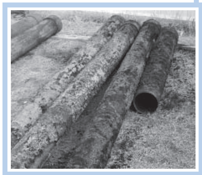
Figure 5. Iron bacteria on pump column riser pipe just removed from a well.
