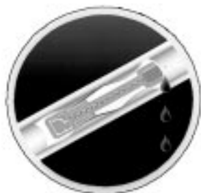
Figure 3. Cutaway example driptape emitter.
