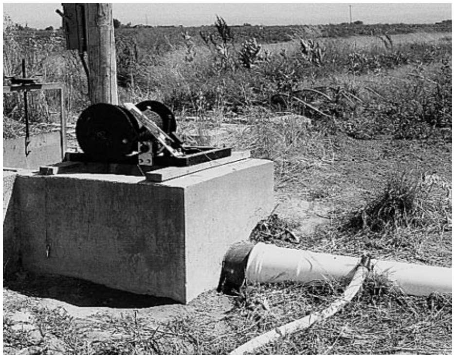
Cablegation gated pipe system. The cable release mechanism is shown mounted on the control box.
