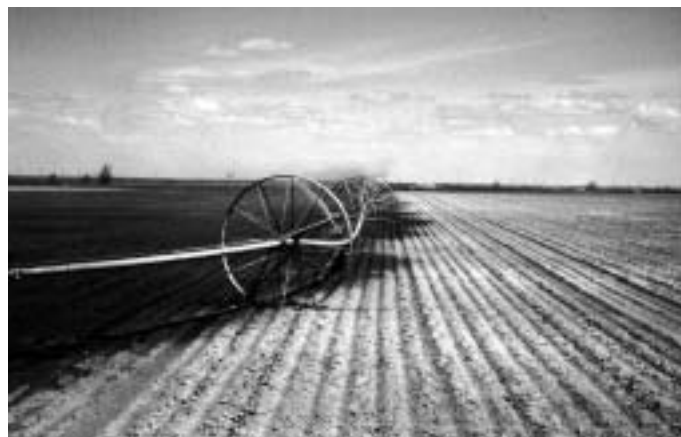
Figure 6. Wind greatly affects the water application pattern from set-move sprinkler system. Here the dark colored soil is wetted and the light colored soil is dry. Wind direction is from right to left.
