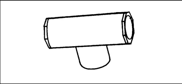
Fig. 12. Compression tee (Comp x Comp x Slip Socket).
