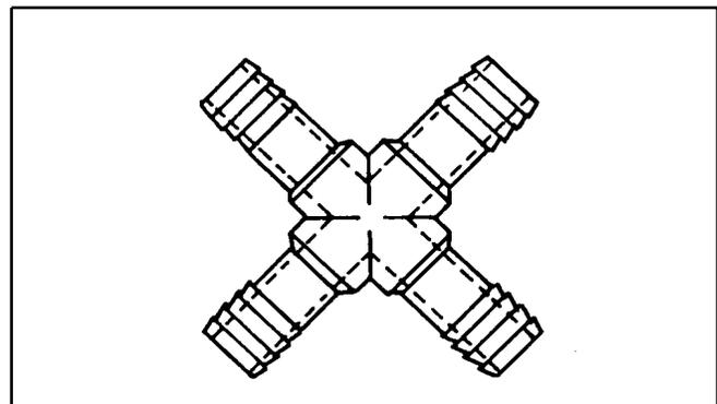
Fig. 5. Insert cross (Ins x Ins x Ins x Ins).
