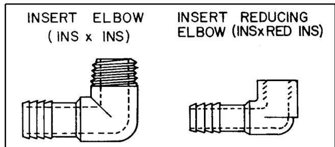
Fig. 6. Cobination elbows.
