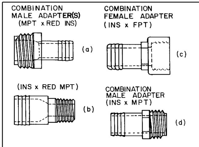
Fig. 1. Insert/comboination adapters.
