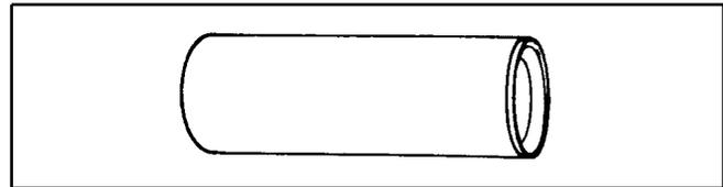
Fig. 4. Compression coupling (Comp x Comp).
