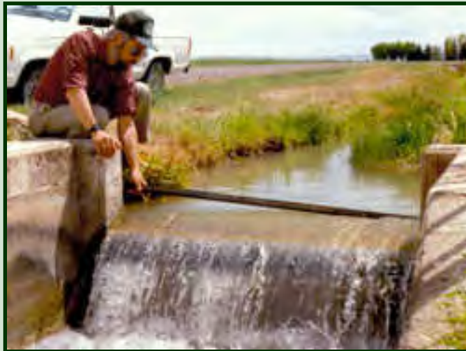
Less turbulence in the flow with angle iron bar raised. Click on image to enlarge.
