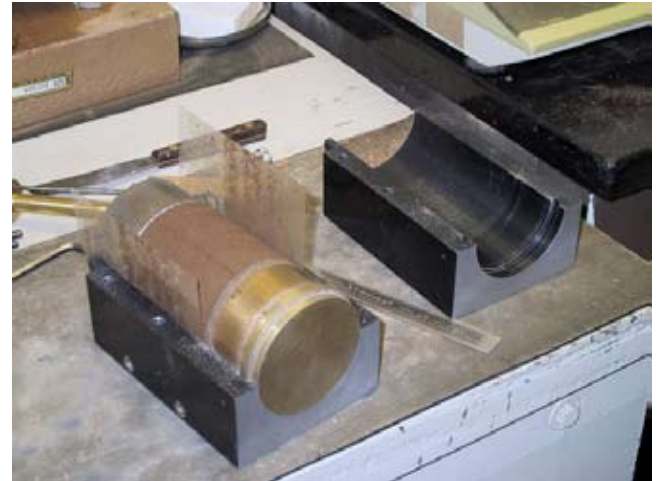
Molded sample after disassembling mold
