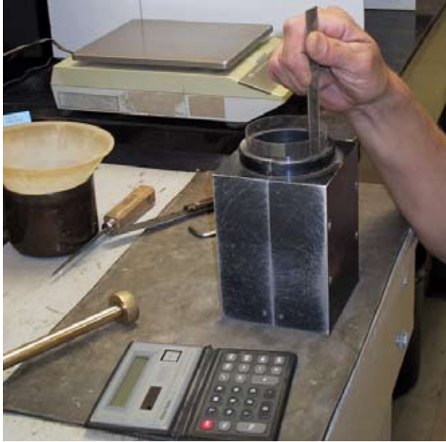
Molding a sample for a flexible wall permeability test
