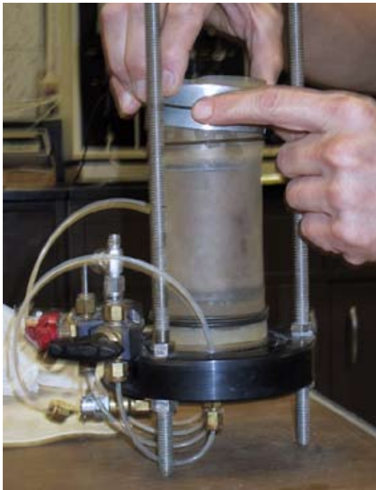
Preparing sample in cell for flexible wall permeability test
