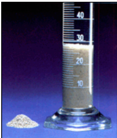
Figure 10D–13 A simple test consists of placing 2 grams of granular bentonite carefully in a calibrated beaker.
