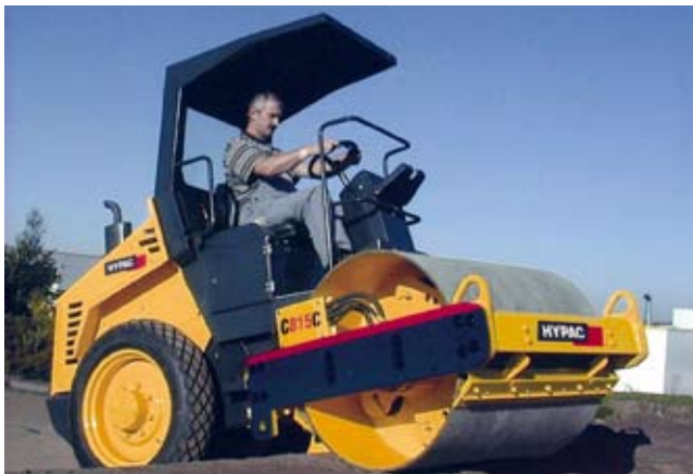
Figure 10D–14 Smooth wheeled steel roller compactor
