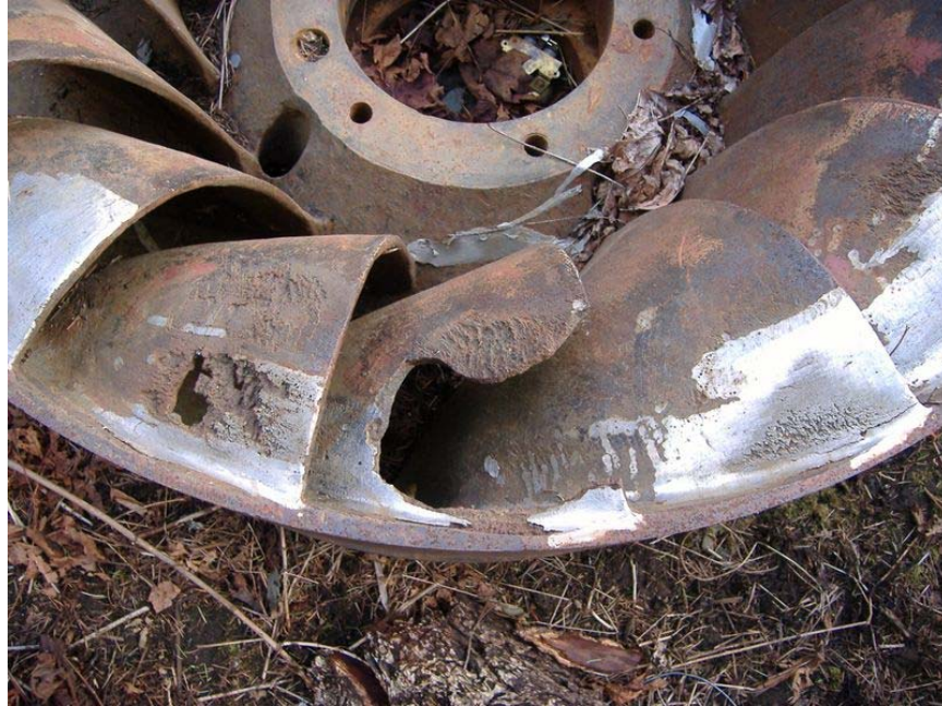
Figure 2. Cavitation damage on the propeller of a Francis turbine.
