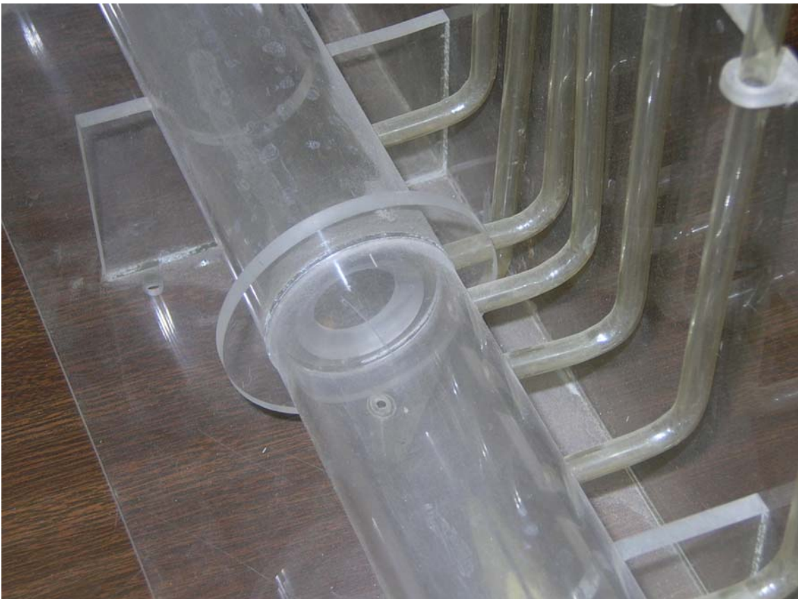
Figure 70. Plexiglas pipe with an orifice meter and piezometric tubes, used in the laboratory to demonstrate orifice flow
