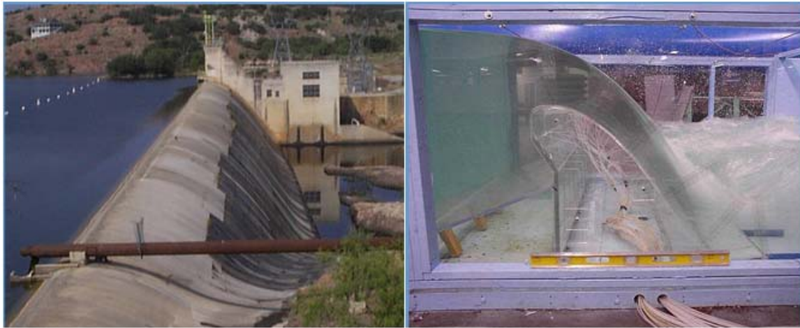
Figure 91. Prototype and model of an ogee spillway (courtesy of the Utah Water Research Laboratory, Utah State University).
