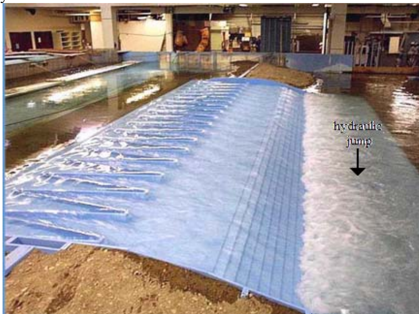
Figure 40. Hydraulic jump observed at the foot of a model spillway (Courtesy of the Utah Water Research Laboratory).
