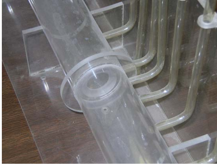
Figure 8. Piezometers near an orifice meter in a pipeline
