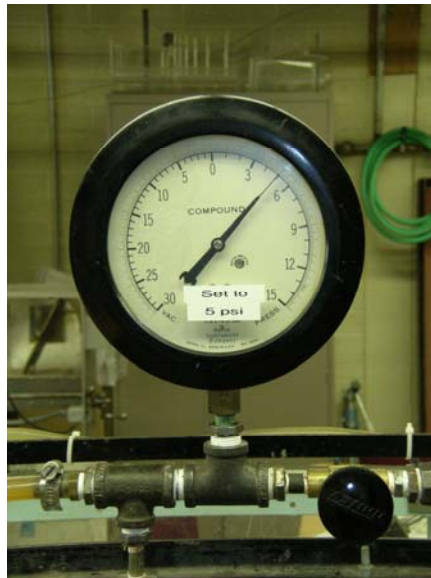
Figure 12. Deformation manometer (Bourdon manometer)
