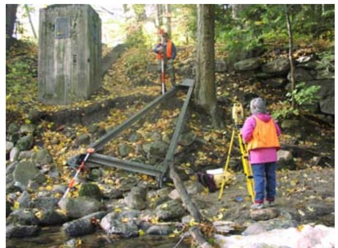
is normal protocol to define a cross section looking downstream with the stationing (in the cross section) increasing from left to right.
