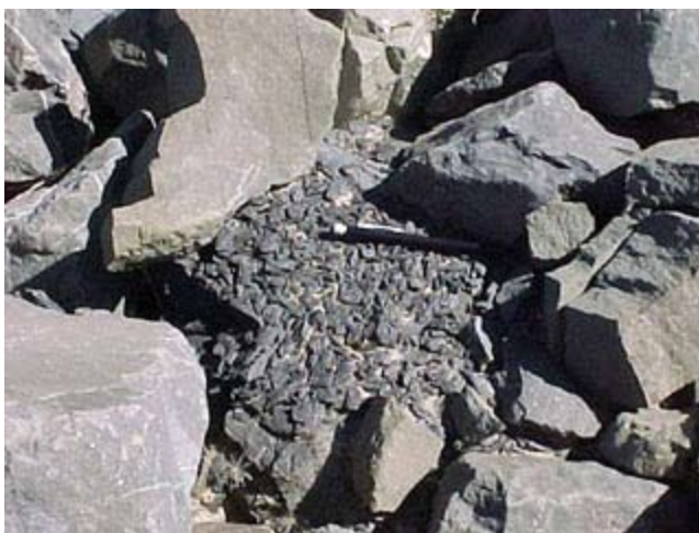
Figure TS14K-1 Capillary breakdown of stone
