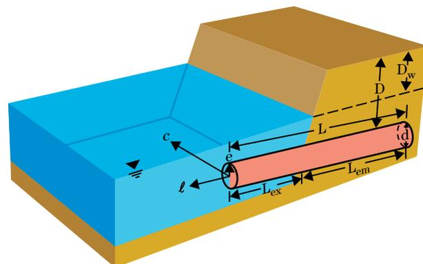
The vertical loading on the log due to the weight of the soil above it will be given by:
