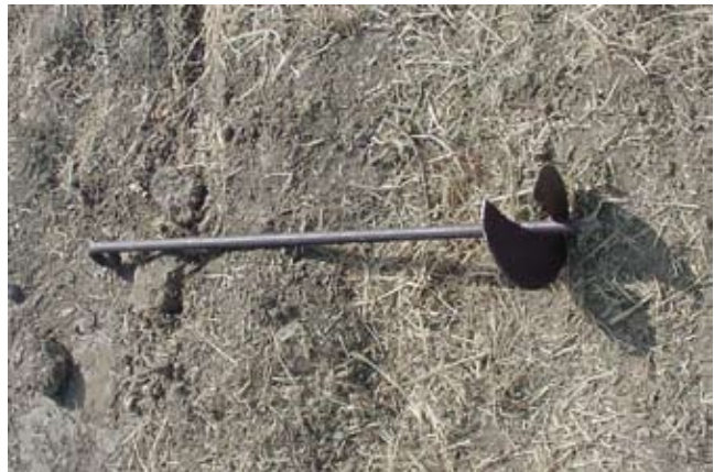
Figure TS14E-7 Screw-in anchor
