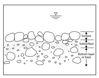
Figure TS13A-4 Coarse bed stream sampling hierarchy
